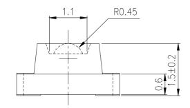
For reflow soldering (propose)
